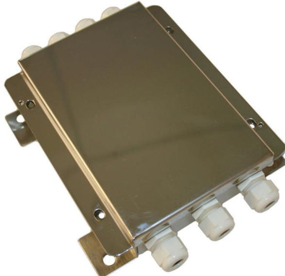
Stainless steel junction box with IP65 protection from water and dust, and fitted with electronic board for junction and equalisation of four or six load cells. Terminal board with screws for easy connection of the load cells and signal adjustment trimmers for accurate and reliable equalisation.
